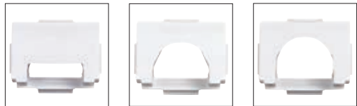
Narrow suction head For better suction at a lower flow rate; use with a variable-speed pump set on low. Medium suction head For use with the majority of suction pumps. Wide suction head Optimises suction at a higher flow rate; use with a variable-speed pump set on high.
